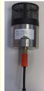
Example of instruments developed to measure n and to retrieve S_A or \rho . On the left, a refractometer called NOSS already tested on profiling floats at 2000 m. Above, a diagram of the device developed in Japan and tested at a depth of over 6000 m (from Ushida et al. , 2019).
