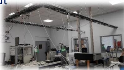
Ten instruments belonging to seven different techniques were challenged with the same formaldehyde gas mixture generated either from a cylinder ( $5.2 \pm 0.26 \mu\text{mol/mol}$ ) or from a permeation system, in different conditions: amount fractions: 2-17 nmol/mol; RH=60%; w/ & w/o  $\text{O}_3$  (50 nmol/mol); ambient air
