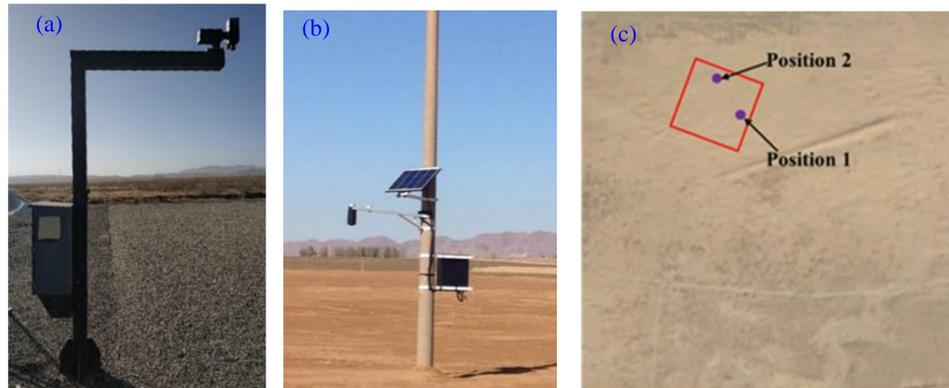
Figure 2. Automatic observation systems of ground reflected radiance in the Baotou site. (a) Observation system on grey target; (b) observation system on sandy site; (c) the positions of the two spectrometers on sandy site.
