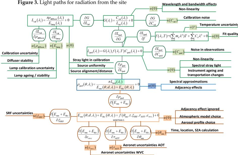
Figure 4. Uncertainty tree diagram for the Baotou measurements of ground spectral reflectance.
