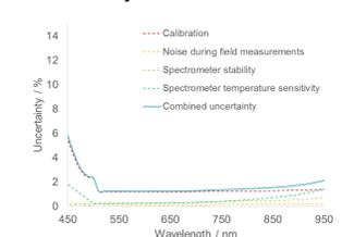
Figure 9. The uncertainty associated with field measurement of radiance
