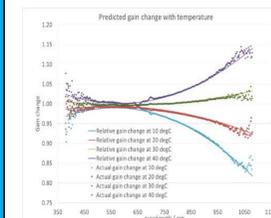
Figure 7. Predicted gain change with temperature
