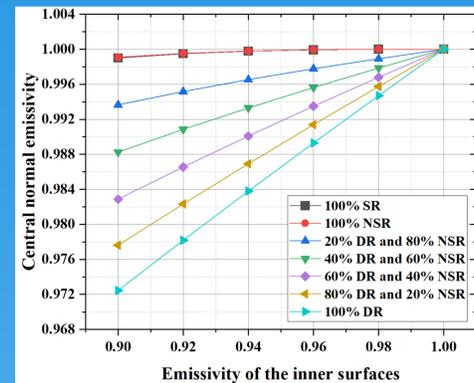
Fig. 3. Normal emissivity at the center of the blackbody with different reflection types.
