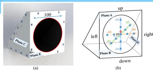
Fig. 2. Model of the blackbody and simulated locations of emissivity.
