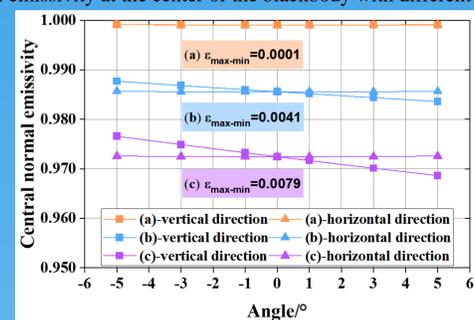
Fig. 4. Central directional emissivity at different angles.
