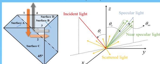
Fig. 1. Optical transmission model and three types of reflected light.
