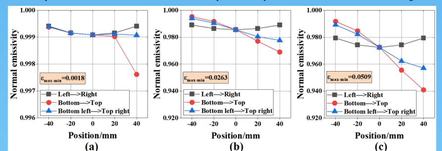
Fig. 5. Normal emissivity uniformity of the blackbody with different surface settings.
